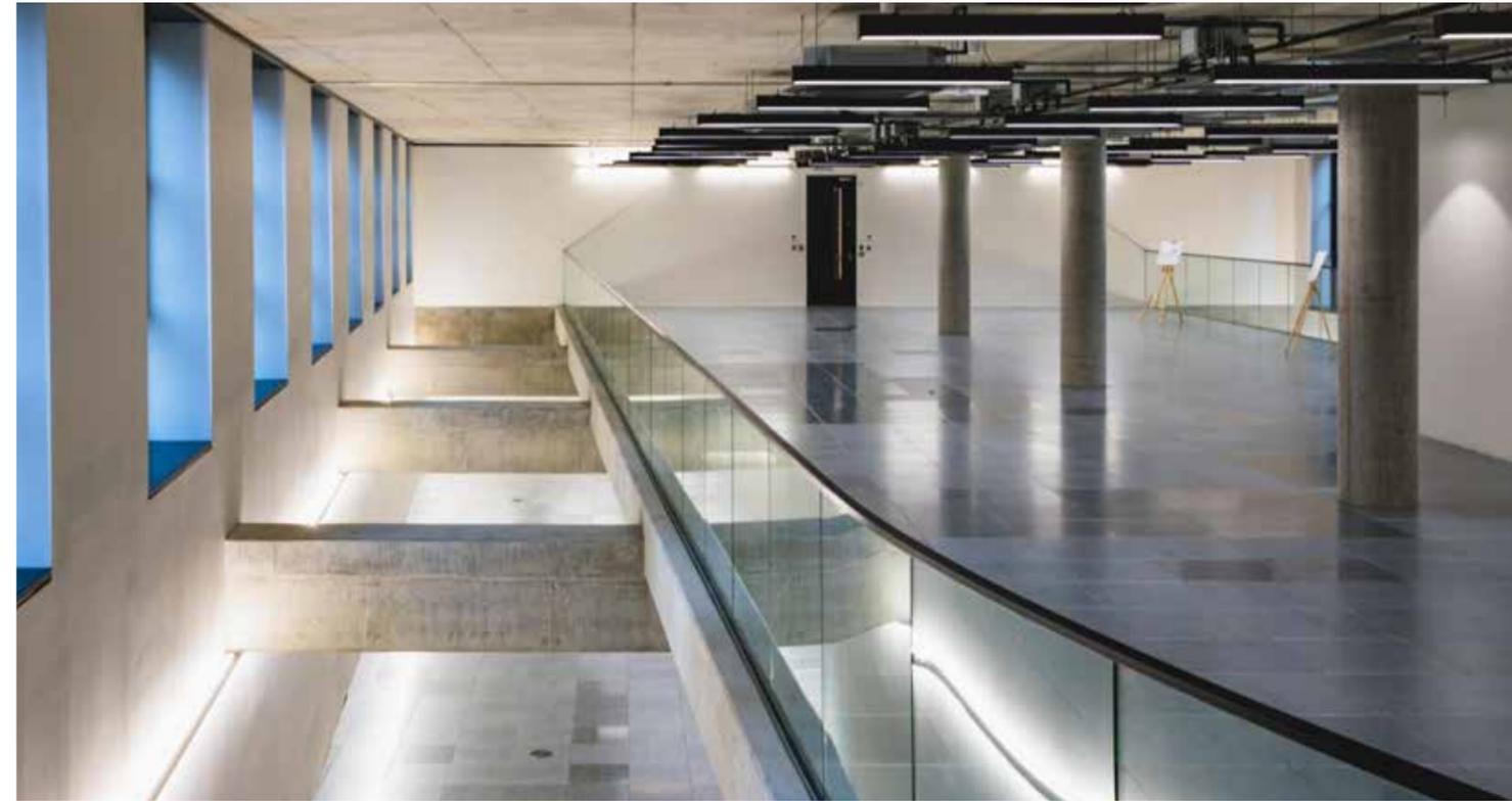
The Phipp Street project saw Glass & Stainless provide some internal glass work for a flexible new office space in Shoreditch, Central London. Frameless channel glass was mixed with curved glass and a curved handrail to create 65 linear metres of internal glass balustrades.
